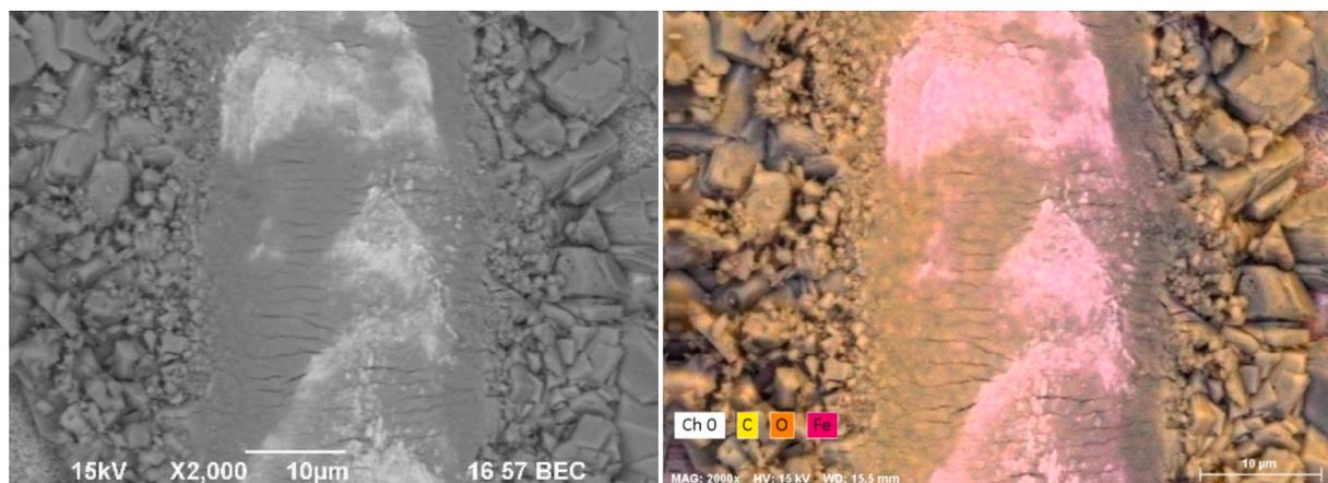
Fig. 17. Left-hand-side: Backscatter image of the critical load detected for iron carbonate at 250 mN of normal force. Bright zones are associated with the exposure of the metal substrate and corroborated with EDS mapping analysis (right-hand-side). Scratch direction: from bottom to top.
